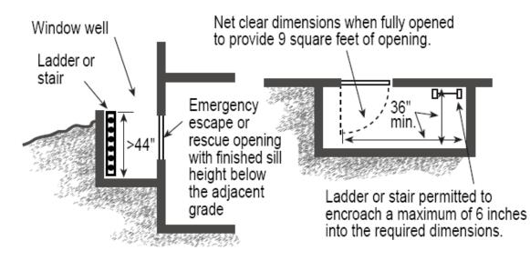
Window wells with a vertical depth greater than 44 inches below the adjacent ground level shall be equipped with a permanently affixed ladder or steps usable with the window in the fully opened position.
